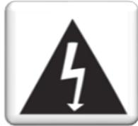
The lightning flash with arrowhead symbol, within an equilateral triangle, is intended to alert the user to the presence of un-insulated 'dangerous voltage' within the product's enclosure that may be of sufficient magnitude to constitute a risk of electric shock to persons. Terminals labelled as
